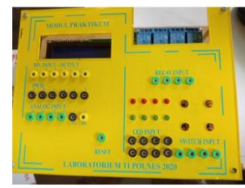
Gambar 20. Alat Peraga praktikum microcontoller Laboratorium TI Polnes
