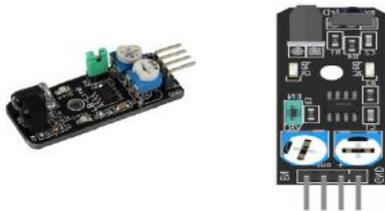
Gambar 8. Modul *Infrared obstacle avoidance* KY-032
