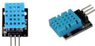
Gambar 6. Modul Suhu dan Kelembaban KY-015(KY-015 Combi-Sensor Temperature+Humidity - SensorKit X40 Wiki, n.d.)
